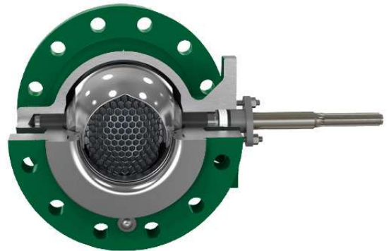
The hexagonal shape holes also offer more drag with sharp corners and more surface area with long flow passage which help slow the process flow to reduce cavitation.
