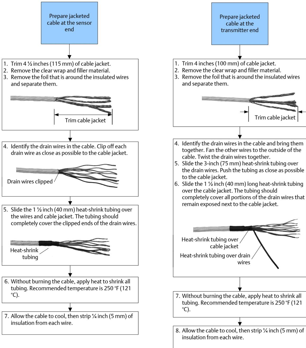
**Figure 4-4: Preparing shielded or armored cable**
