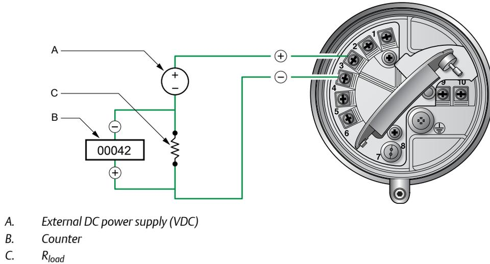
Figure 8-7: Safe area frequency output/discrete output load resistance values
