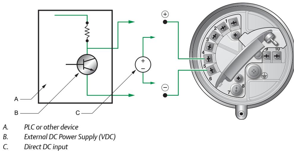
Power is supplied by either a PLC/other device or by direct DC input.
