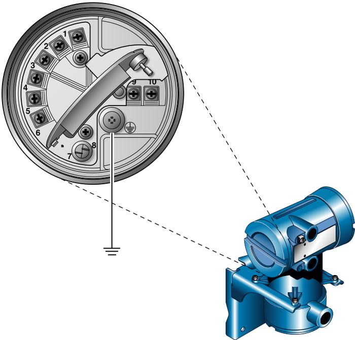
**Figure 4-20: Transmitter external ground screw**
