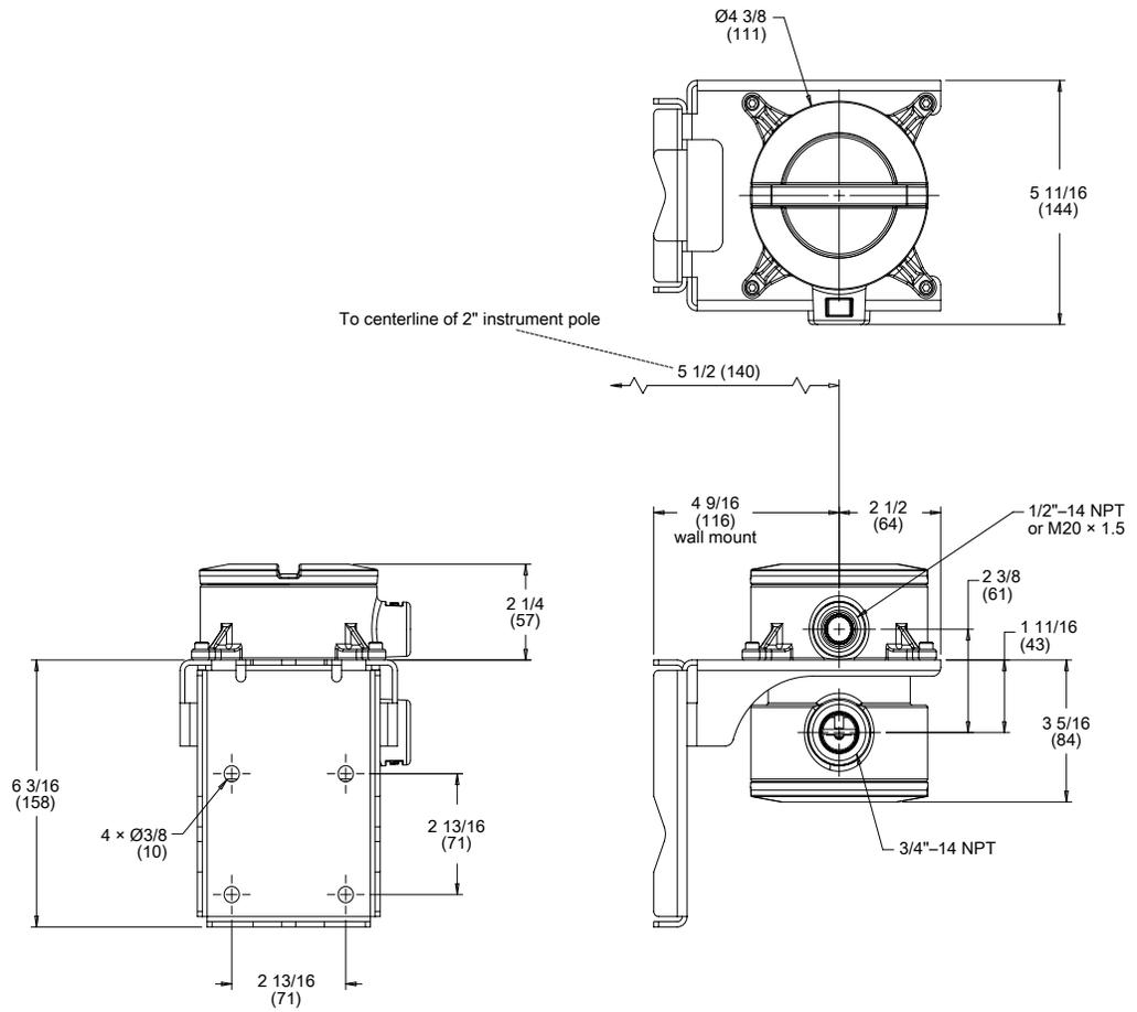
Figure 11-5: Remote enhanced core processor dimensions
