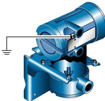
3. Ground the remote core processor according to applicable local standards, using the remote core processor's internal ground screw.
