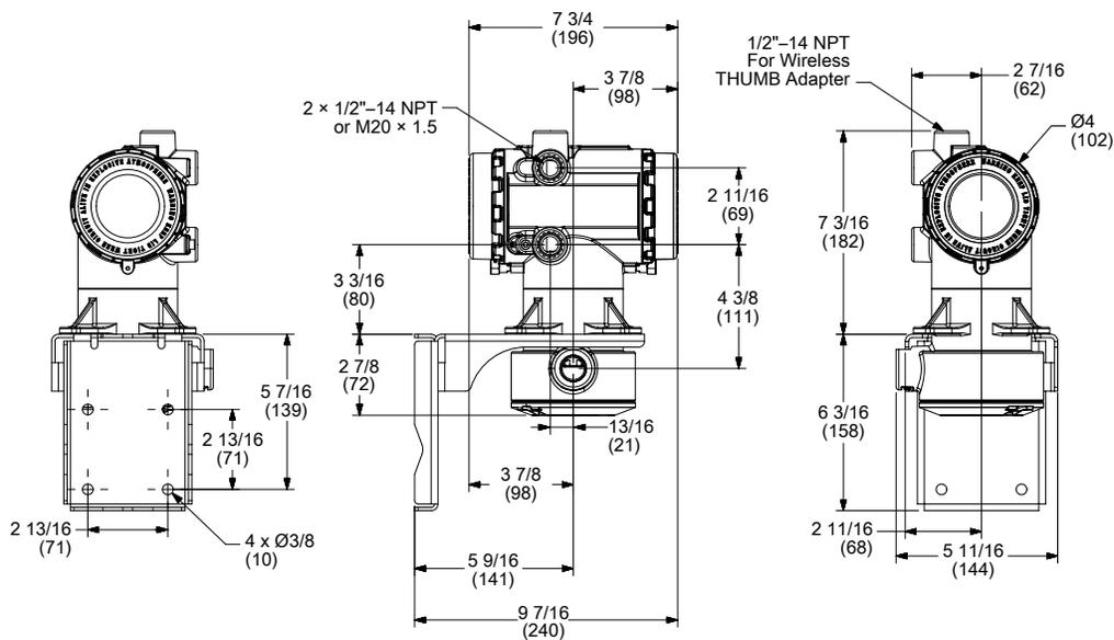
**Figure 11-4: Remote core processor dimensions**
