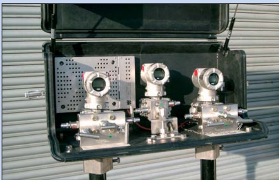
IEX3 Enclosure with heating system
