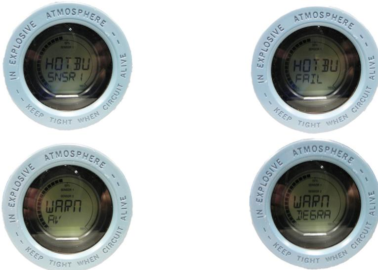
After the sensor has been repaired or replaced, the LCD display on the transmitter will display a message WARN HOT BU, reminding you that Hot Backup is still active, as well as the normal output of the average temperature. The warning message will clear after you have reset Hot Backup. It is recommended that Hot Backup be reset immediately after repairing or replacing the damaged sensor. See “Reset Hot Backup: Fast Keys 2-2-4-1-4” on page 76.
