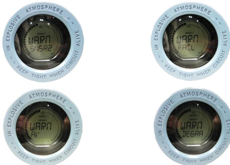
After the sensor has been repaired or replaced, the LCD display warning message will clear and display the output of the primary variable.
