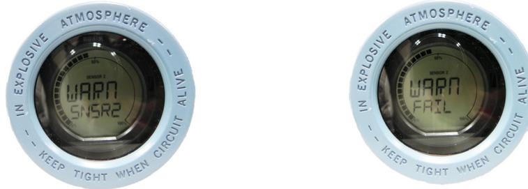
After the sensor has been repaired or replaced, the LCD display warning message will clear and display the output of the primary variable.
