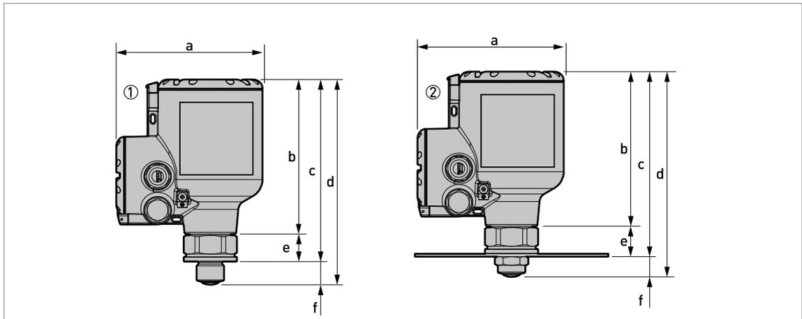
Figure 2-15: DN20 / 3/4" Lens antenna versions
