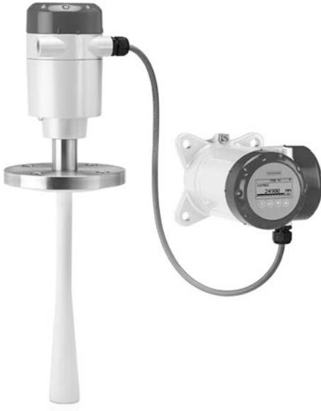
This 10 GHz 2-wire FMCW radar level transmitter measures distance, level, volume, mass and flow rate of liquids and pastes. It is ideal for corrosive products with its PP or PTFE antenna options. It features unique PP and PTFE antennas for aggressive products. The device is able to measure distances up to 30 m / 98.4 ft in process conditions up to +250°C / +482°F and 40 barg / 580 psig.
