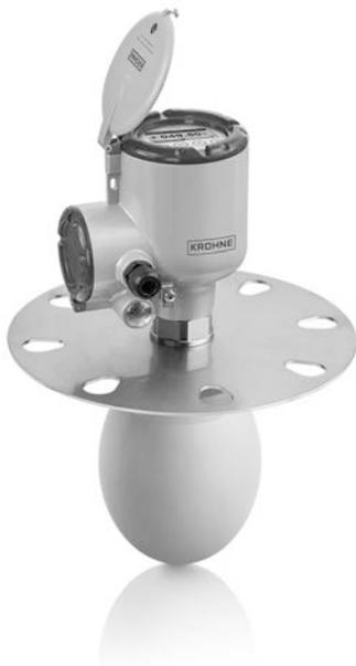
By combining high signal dynamics and FMCW radar technology, this market-entry 24 GHz radar device measures accurately and reliably the level of solids like stone, plastic granulates or coffee beans. No need for expensive antenna aiming kits or purging systems; the proven Drop antenna design minimizes scaling and is not affected by the angle of repose.
