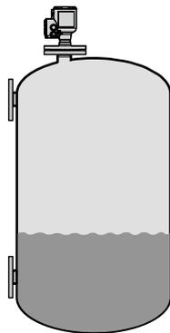
The level transmitter can measure the level of a wide range of liquid products on a large variety of installations within the stated pressure and temperature range. It does not require any calibration: it is only necessary to do a short configuration procedure.
