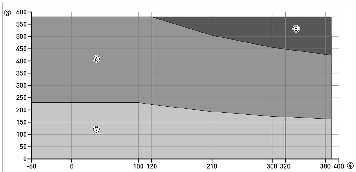
Figure 2-14: Pressure / temperature de-rating (ASME B16.5), flange and threaded connections, in °F and psig
