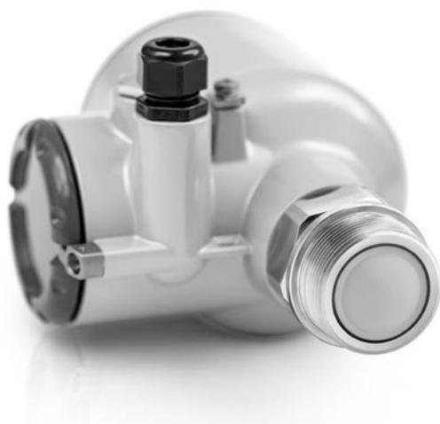
The small beam angle and negligible dead zone of this 80 GHz FMCW radar level transmitter makes it the premium choice for liquids in small and narrow tanks with internal obstructions like agitators or heating coils, as well as tanks with long nozzles. It can even measure through tank roofs made of non-conductive material (e.g. plastic, fiberglass or glass). The flush-mounted PEEK Lens antenna (no tank intrusion) is insensitive to deposit.
