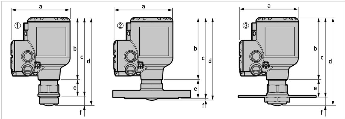
Figure 2-17: DN40 / 1½" Lens antenna versions
