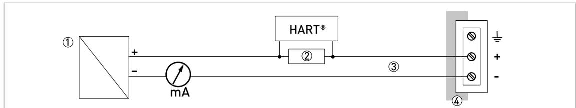
Figure 4-3: Electrical connections for non-Ex devices
