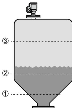
A strapping table function is available in the configuration menu for volume or mass measurement. Up to 50 volume (mass) values can be related to level values. For example:
