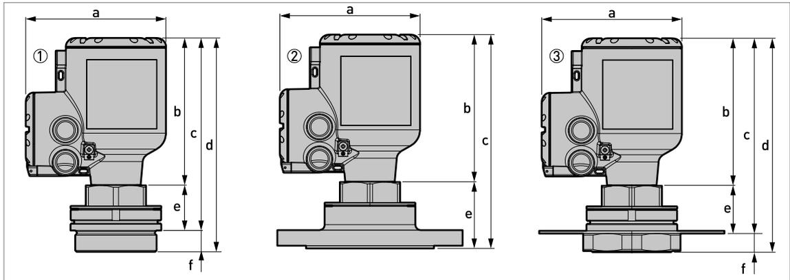
Figure 2-18: DN70 / 3" Lens antenna versions
