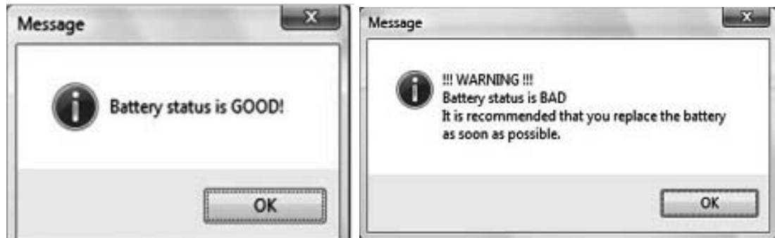
Figure 13 Configurator good and bad battery indicator
