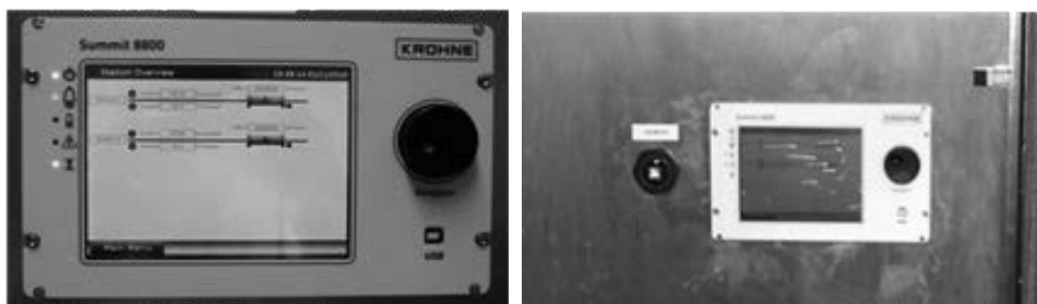
Figure 7 Panel mounted installations
