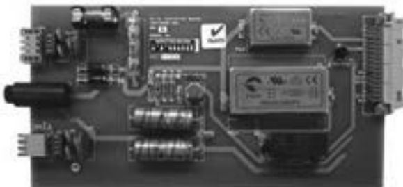
Figure 24 Power supply unit
