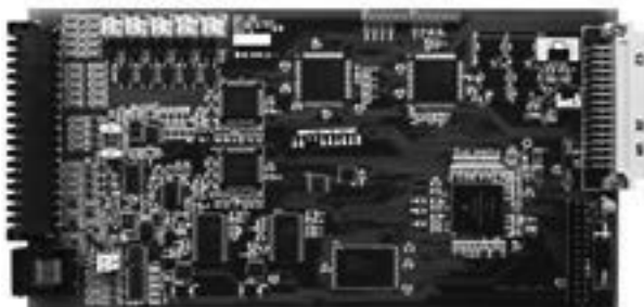
Figure 28 Typical I/O board
