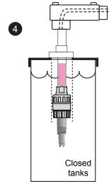
The Signet pH/ORP electrodes are designed to install in tanks by attaching conduit to the  $\frac{3}{4}$  in. (ISO 7/1-R  $\frac{3}{4}$ ) threads at the top of the accompanying preamplifier or sensor electronics:
