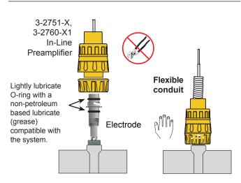
Signet Installation Fitting DN15 to DN100 (½ in. to 4 in.)
