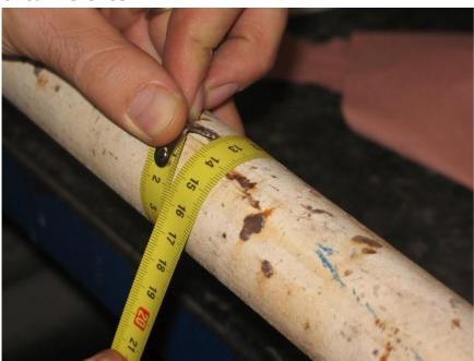
6. Measure the pipe's thickness.
