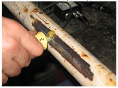
Now place the Thickness Gauge TT100-TM8812-NG sensor and measure the pipe's thickness:
