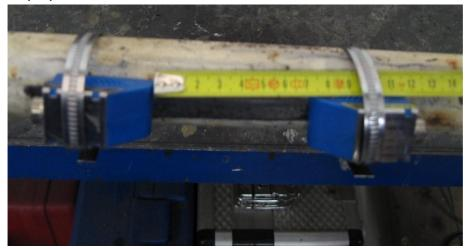
11. Now the clamp-on sensors installation is complete:
