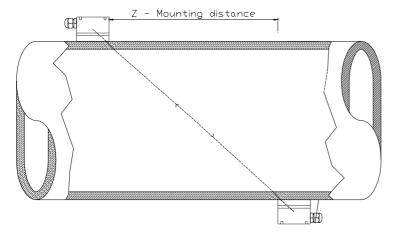
"Z" mounting is more complicated than "V" mounting and it is necessary to create a band of foil as long as the pipe circumference and as wide as indicated in window 25. Additionally, add a piece of paper to wrap the pipe.
