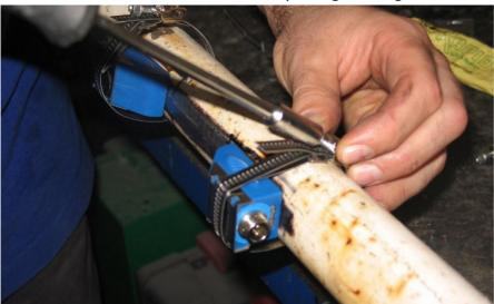
10. It is necessary to install the sensors according to the distance value the device displays in MENU 25:
