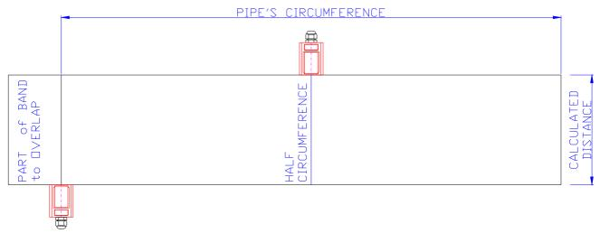
Once the fascia is fixed onto the pipe's circumference (with adhesive tape), it is possible to fix the sensors, as shown in the picture. If the pipe is horizontally mounted, it is suggested to mount the sensors as shown in the next picture. If the pipe is vertically mounted, refer to the instructions of "V" mounting method.
