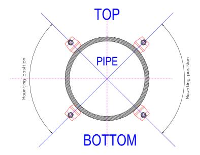
In case of vertical mounting, avoid installing the transducers on downward pipe walls, even if they are under pressure. The pipes with an external lining such as tar, polyethylene, epoxy, should be cleaned when in contact with the transducers.
