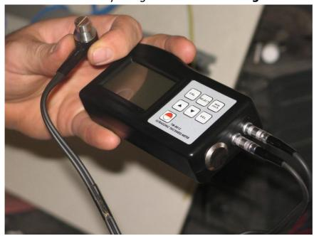
Before using the Thickness Gauge sensors, please remember to use the coupling grease:
