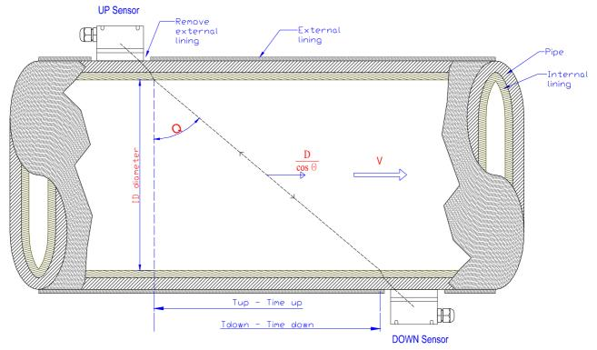
The measures are taken by 2 sensors in direct contact with the pipe's external surface.
