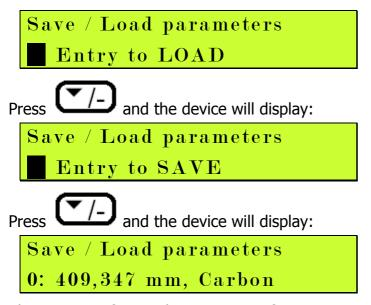
This setting refers to the just set configuration: DN400 carbon steel pipe.
