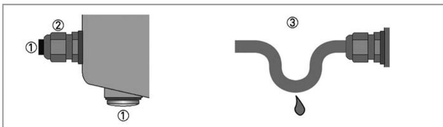
**Figure 4-8: Cable feedthrough**
